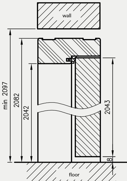
required height of the wall opening 2097 mm
