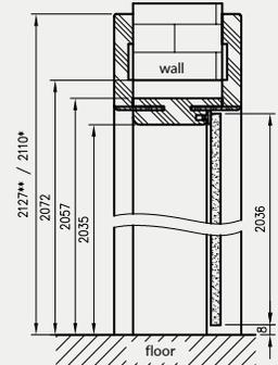
required wall passage height 2066 mm (2072 mm for glass doors)
