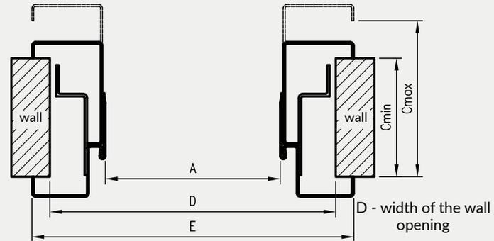
\* - with the use of a steel threshold - the actual height of the door frame passage will be reduced by 20mm from the floor
