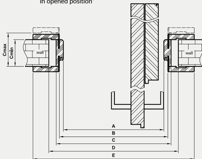
\*NOTE: When doors are fully opened, the door fittings slightly reduce the clear opening by approx. 10 cm. (this value doesn't take into account door handle)
