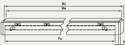
Masking strip and guide bar for double sliding system is made by connecting two elements of single system.
