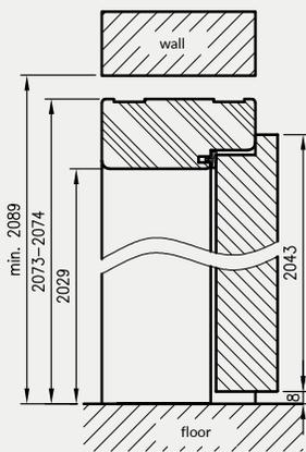
required height of wall passage 2089 mm (2095 mm for glass doors)
