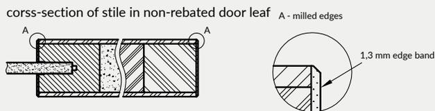
VETRO collection glass panes have obverse and reverse sides (important in juxtaposition of doors opening inversely). Presented horizontal cross-sections shows the arrangement of glass pane in the obverse version. When choosing a reverse version, glass pane is rotated by 180° around the vertical axis.
