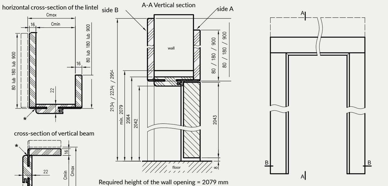
\*NOTE: 075-095 door frame has a different cross-section, shallow milling for architrave, for a 75-89 mm wall thickness, it will be necessary to shorten pen of the architrave element.
