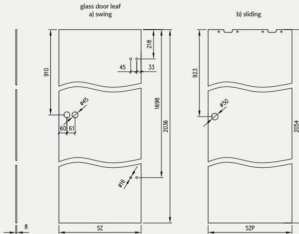
Door leaf unit is made of safe, plain or glued, tempered 8mm glass pane which has in standard option holes for assembly of:
