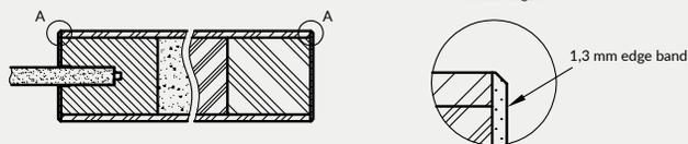
VETRO collection glass panes have obverse and reverse sides (important in juxtaposition of doors opening inversely). Presented horizontal cross-sections shows the arrangement of glass pane in the obverse version. When choosing a reverse version, glass pane is rotated by 180° around the vertical axis.
