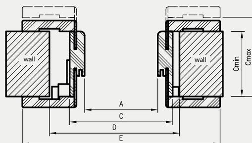
\*NOTE: 075-095 door frame has a different cross-section, for a 75-89 mm wall thickness, it will be necessary to shorten pen of the adjustable angle element.
