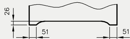
Use of ventilation undercut in door leaf unit with width "80" - "90" and standard clearance between door leaf and floor (8mm) will fulfill ventilation requirement - total ventilation surface 0,022 m<sup>2</sup>.
