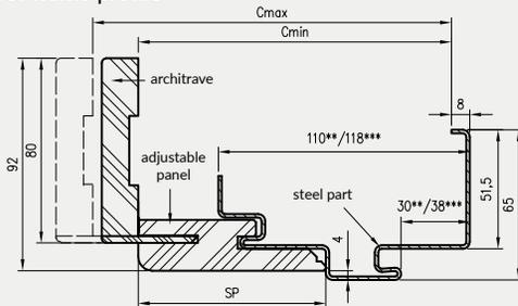
For a specific wall thickness, select the appropriate option of the adjustable panel with an architrave (Cmin)
