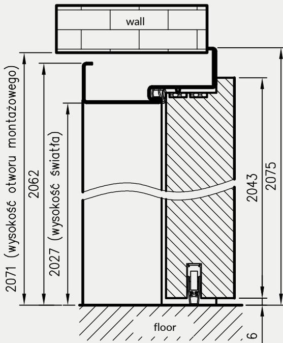
horizontal cross-section of door frame mounted in the wall
