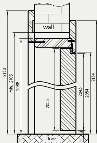
Required height of the wall opening = 2103 mm
