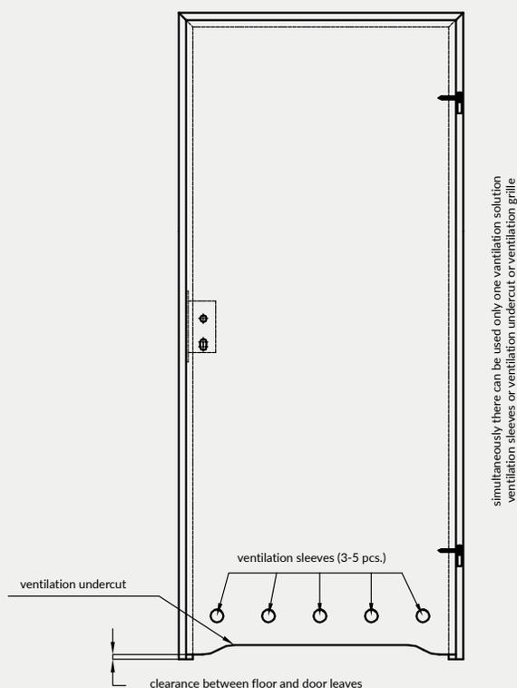
The above - stated required clearance height of the space under the door assures total ventilation surface of 0.022 m<sup>2</sup>. The standard clearance for door leaf is 8mm high.
