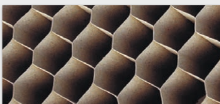
(A) stabilising insert "honeycomb"
