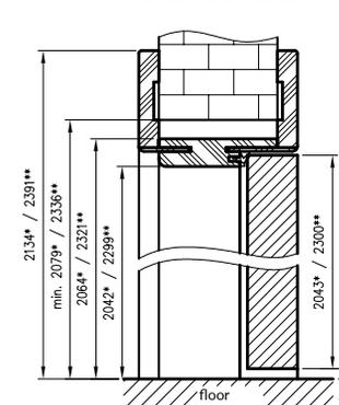
required height of the wall opening 2079\* / 2336 mm\*\*
