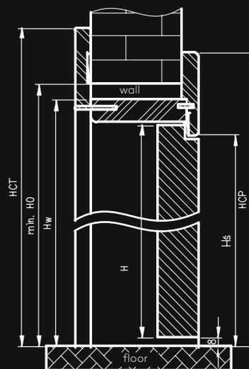
Adjustable door frame with inverted rebate is made of high-quality wood-based board. From the display side, the door frame is covered with MATT foils, CPL laminate or painted with the highest quality acrylic UV varnishes. To ensure high quality of painted door frames, they are covered with a special material that forms a uniform base before painting. Its construction is adapted to the leaf thickness of 40 mm and can be assembled on walls with a thickness of 90 - 290 mm...
