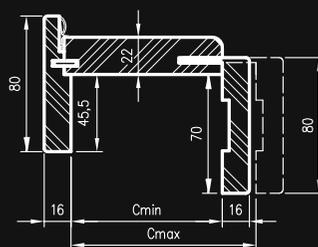
vertical cross-section of adjustable inverted rebate door frame
