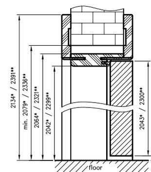
required height of the wall opening 2079\* / 2336 mm \*\*
