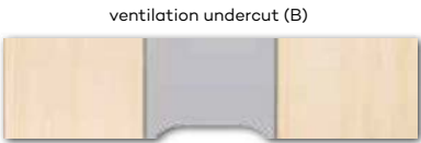
VETRO B - doesn't fulfill ventilation requirements
